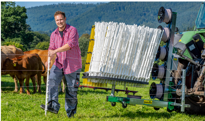
Exchangeable magazine for up to 400 posts
